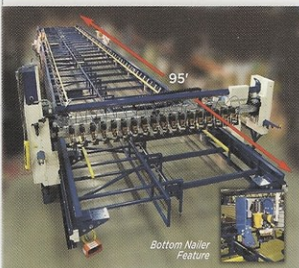
76 feet of Expanded Wall Opportunity required a "custom built" wall table with optional Dual Beams & Plate nailing tool carriages.
